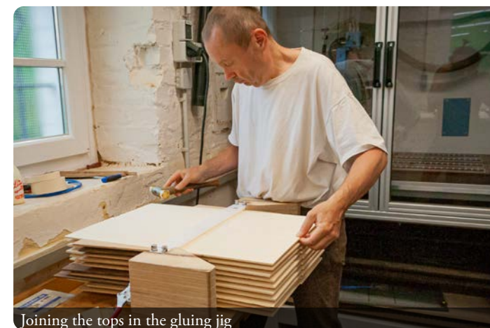
Joining the tops in the glueing jig
