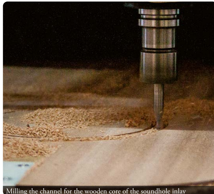
Milling the channel for the wooden core of the soundhole inlay
