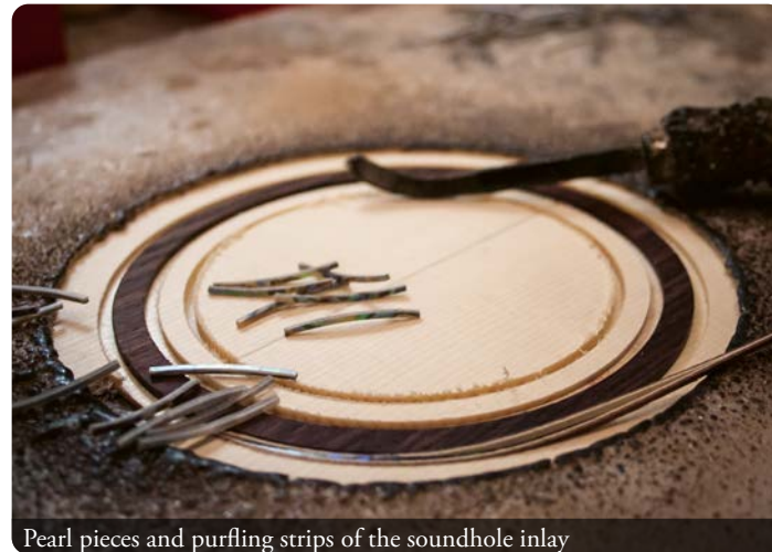
Pearl pieces and purfling strips of the soundhole inlay
